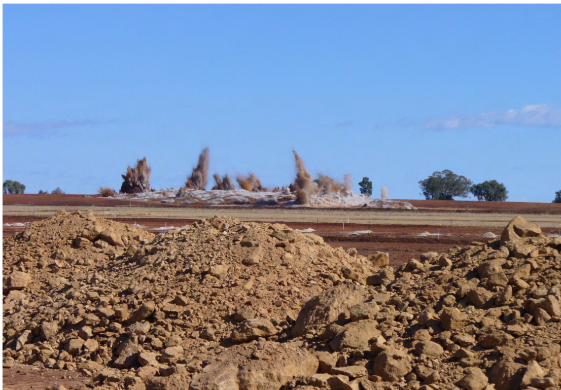
Plate 8 - Blast for Box Cut - May 2008
